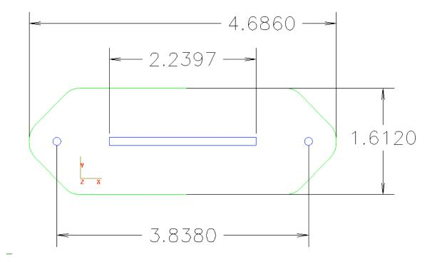
$V\ V\ G$  blade Dogear pickup dimensions {all dimensions in inches]; the pickup requires a cavity  $\sim 0.700"$  deep.
