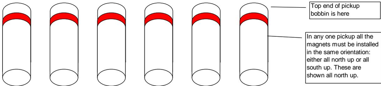
My usual convention for the magnetic orientation in a set of three pickups is:
