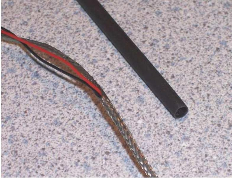
I use a hot air gun (intended for stripping paint) to shrink the shrink wrap. Once heated the shrink wrap will be snug around the cable as shown in the photo below:
