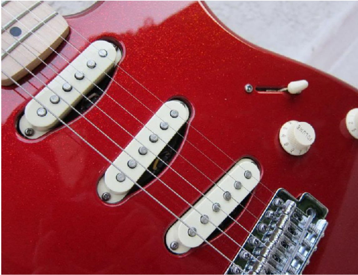
Figure 2. Pickups direct mounted to the body of the instrument. Each of the three pickups is secured to the body of the instrument using three wood screws. Tubing or springs can be used under the pickups at the location of the mounting screws and compressible foam can be placed under each pickup at the bottom of the pickup cavity. Rotating these mounting screws clockwise will lower the pickups.
