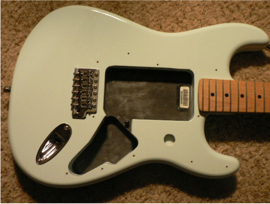
Figure 3. Strat style instrument with swimming pool route. A pickguard is normally used with this type of pickup cavity route to cover both the large pickup cavity and the controls cavity.
