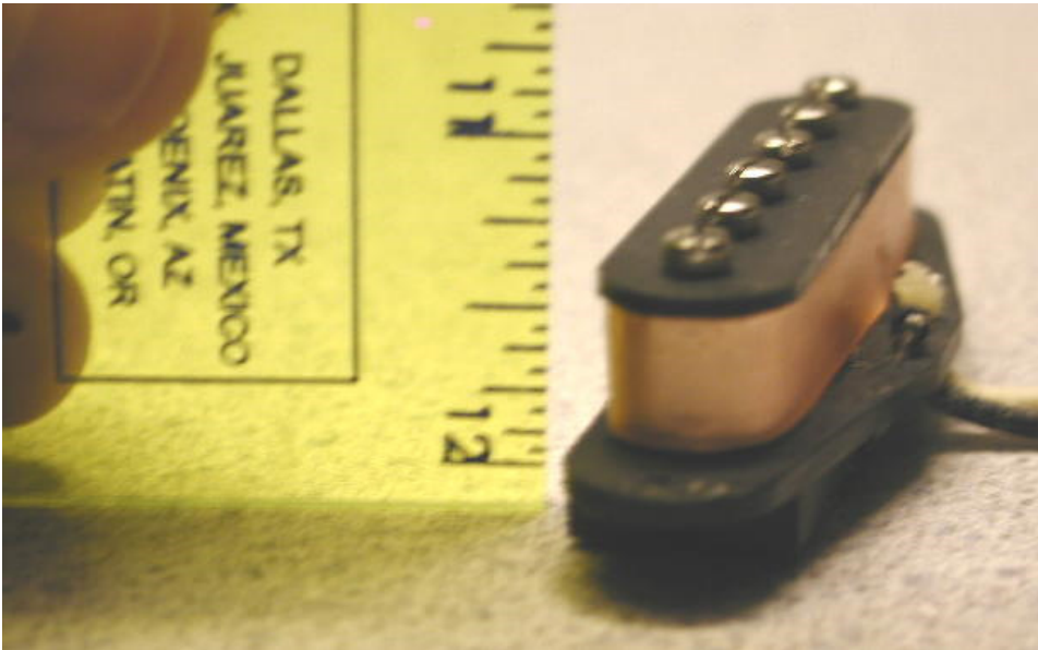
Figure 4. A strat size pickup (Model SP-90) measures just over \frac{3}{4} " tall from the bottom of the bar magnets to the top of the adjustable pole pieces.
