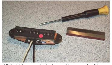
6.Re-install the cover using the three machine screws. Carefully store the original magnets.
