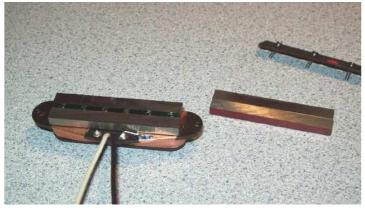
5. Make sure the two magnet bars of the new magnet assembly are aligned with each other and the orientation is correct.
