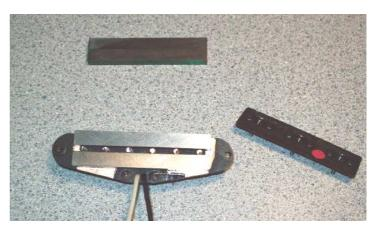
2. Remove the magnet cover plate and set aside; carefully pry the magets from the base of the pickup. Note magnet orientation.
