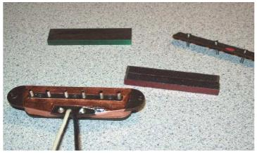
3. Remove the black tape from the original magnets and transfer to the new magnets.
