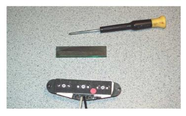
1. Access the back of the SP-90 pickup and use a small Phillip's drive screwdriver to remove the three machine screws on the bottom.
