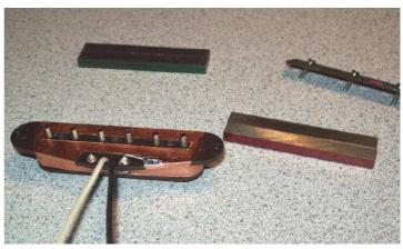
4. The new magnets will be installed with the black tape between the magnet and the botttom of the pickup body.
